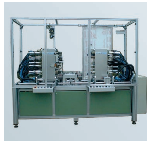
23 placing heads to assemble a computer chassis
